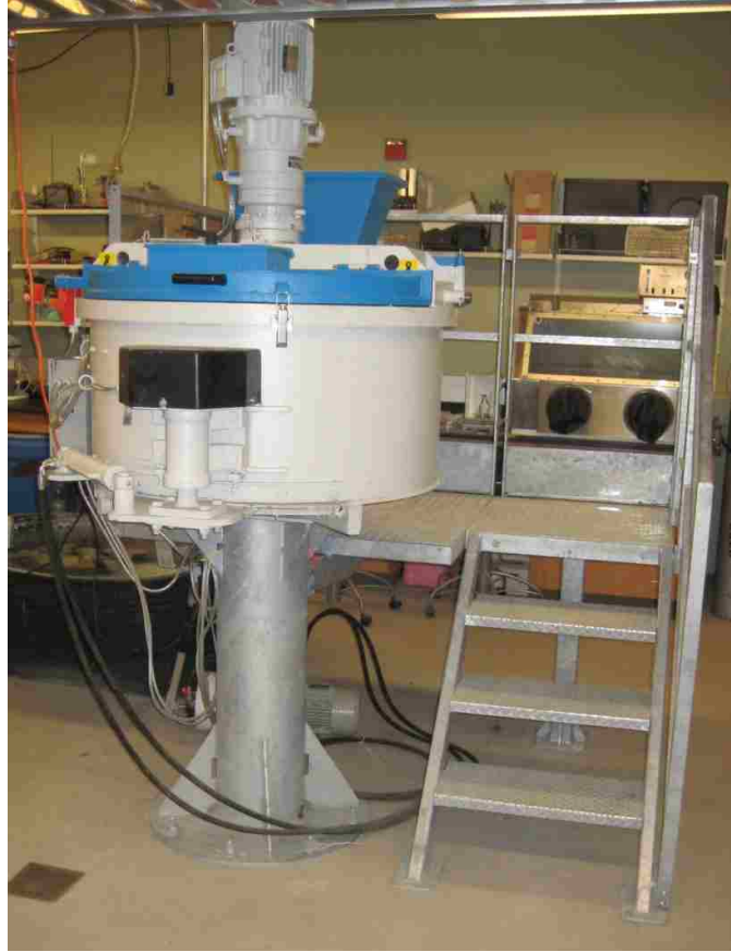
Figure 3.24: Sicoma planetary shear mixer used for producing UHPC
