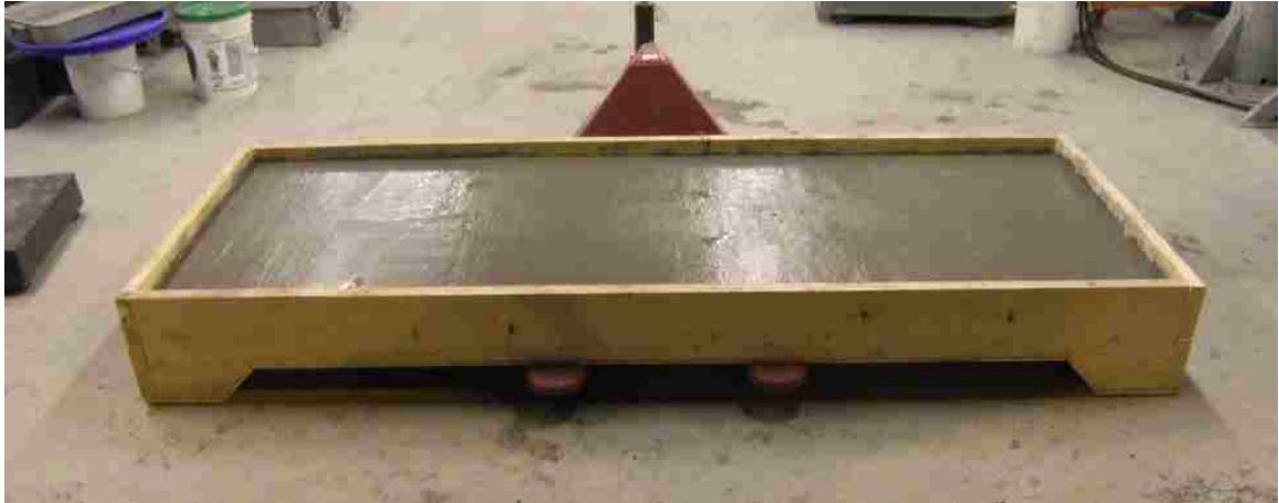
Figure 3.15: The finished control slab
