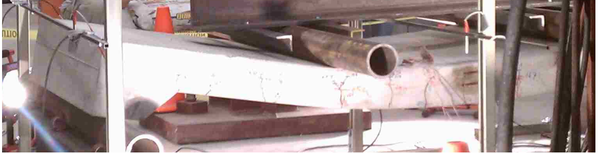
Figure 5.2: Deflection of the control slab near failure
