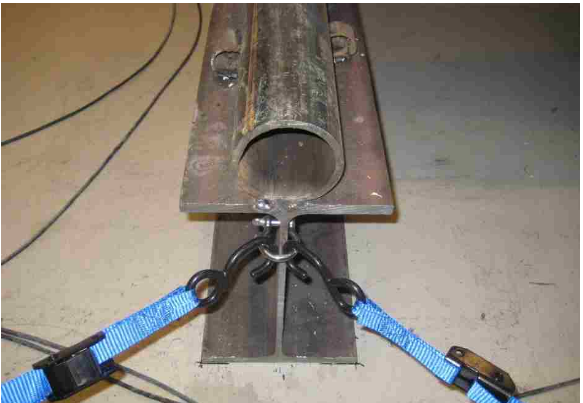
Figure 3.7: Tie Down Connection for Increased Stability
