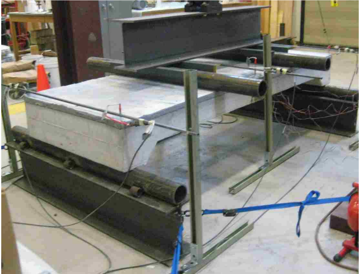
Figure 3.34: The strengthened slab prior to testing
