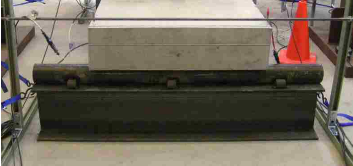
Figure 3.5: The Pinned Connection
