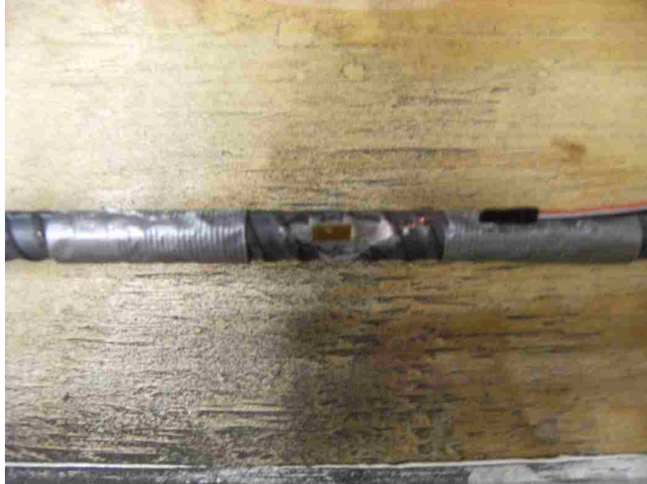
Figure 3.16: Strain gauge on a reinforcement bar
