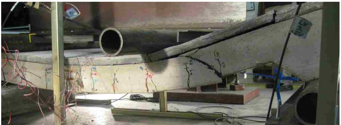
Figure 5.24: Shear failure in the NVC
