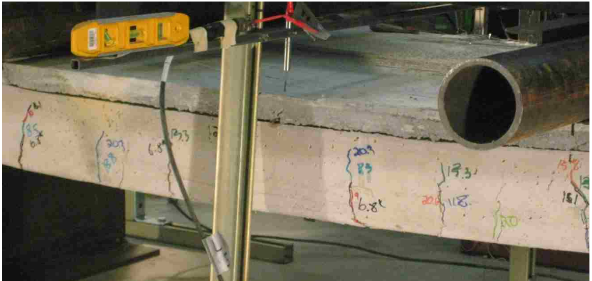
Figure 5.15: Strengthened slab after UHPC debonding
