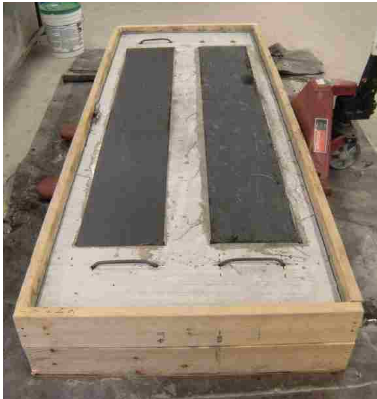
Figure 3.23: CFRP and shear-friction reinforcement
