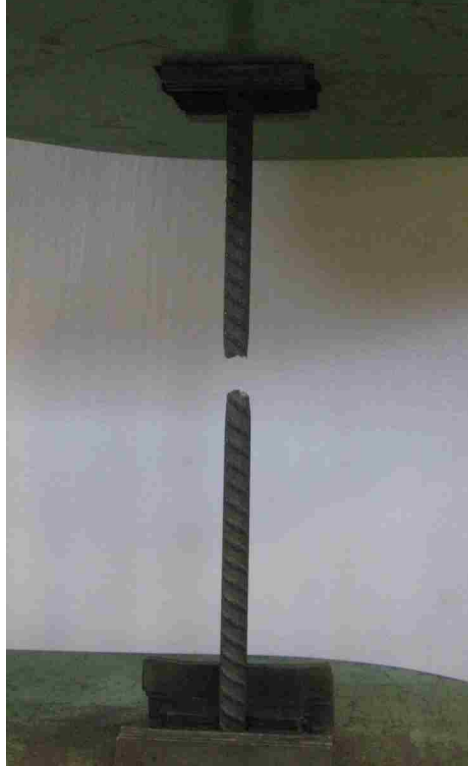
Figure 3.30: Direct tension test of the flexural steel
