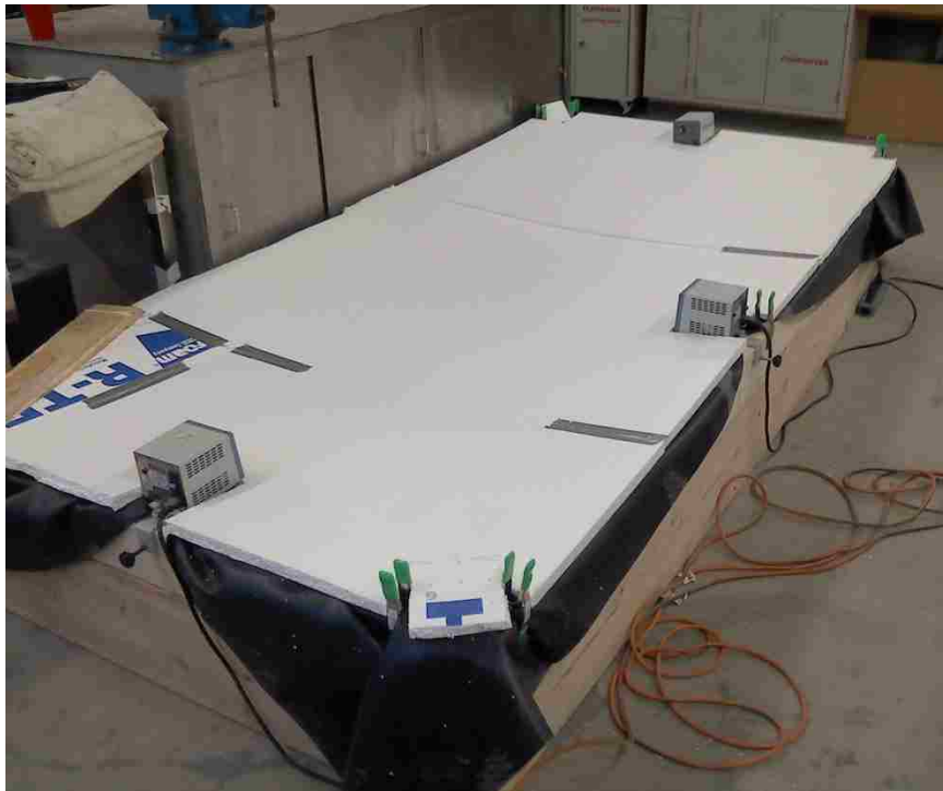
Figure 3.28: UHPC curing tank
