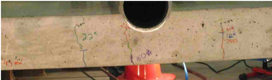
Figure 5.1: Cracks developing in the control slab
