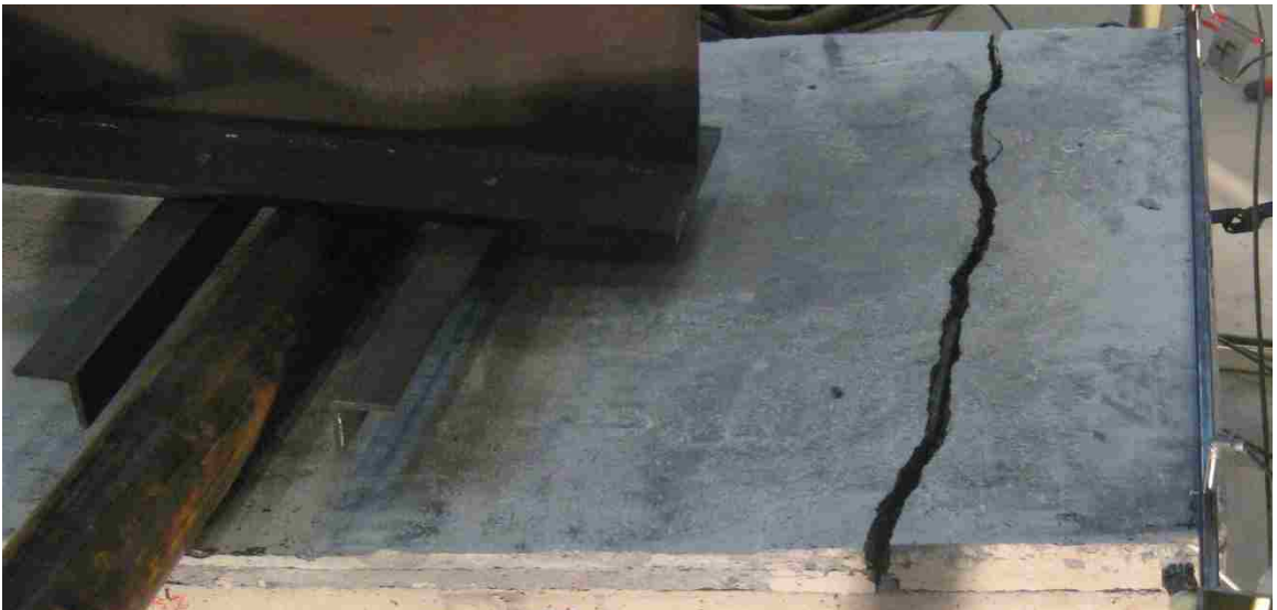
Figure 5.17: Horizontal shear failure of the UHPC overlay outside of the shear-friction reinforcement (plan)
