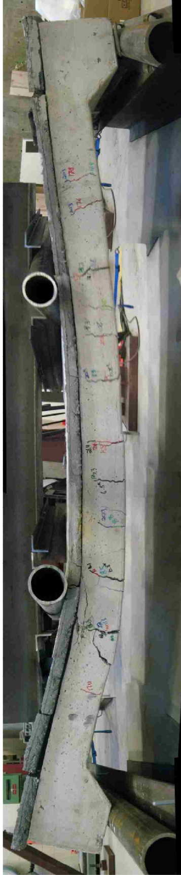
Figure 5.20: Profile of the strengthened slab at failure
